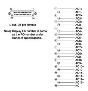
The analog output signals of the instrument are not isolated individually. It is recommended to isolate the signals individually to eliminate the interference from unwanted signals or other external interference, especially if the cable exceeds 30 meters or leads to outdoors.
